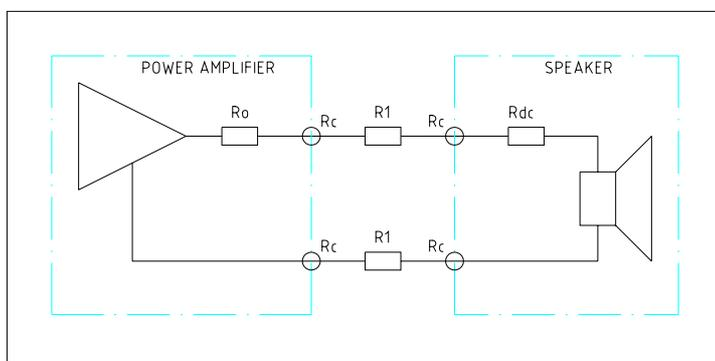
*Example of total resistance between power amplifier and loudspeaker.*
